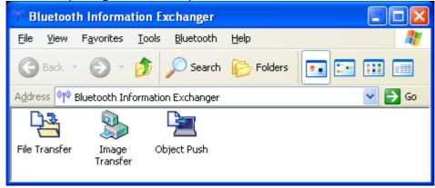
Double click the "Image Transfer" ICON to perform any BIP operation to a remote device
