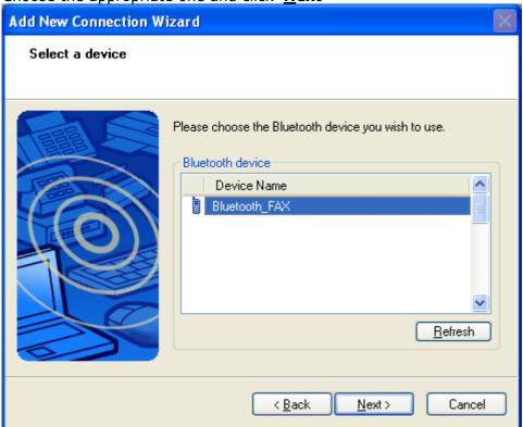
Now a service search will be performed and checked whether security is required by one of the Bluetooth<sup>™</sup> devices. In that case <u>pairing</u> will be done. You have to know the <u>Passkey</u> of the remote device.
